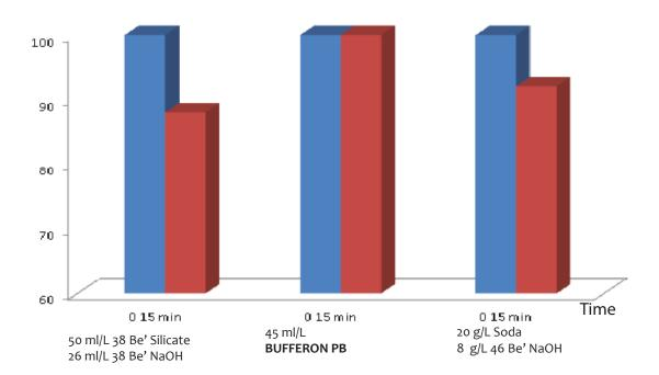
Graphs display that, in case of NaOH / Silicate, all recipes are failed. In case of NaOH / Na2Co3, only light shades are stable and others are failed.
