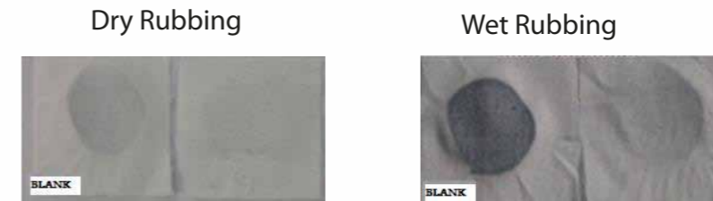
Reactive Black Dyeing, 40 g/L ABRASION EXE
